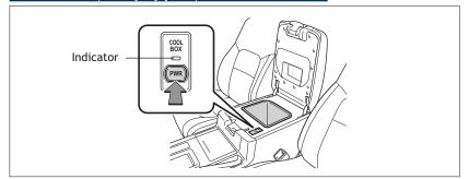
Push "PWR" button to turn cool box ON; indicator light will illuminate.
